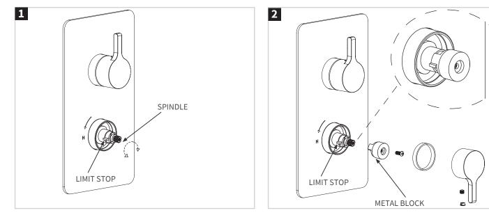
Remove the temperature control handle, metal block. Rotate the exposed thermostatic spindle (clockwise for cold, and anti-clockwise for hot), until the maximum desired showering temperature is set. The suggested maximum pre-set temperature is 42°C. Without any move at the spindle, replace the metal block so that limit stop up to the right hand side of the limit stop on the cartridge. Then refit the temperature control handle.
