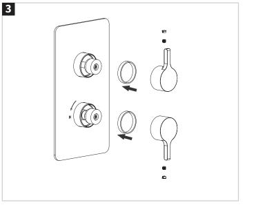
Assemble the handles and the plastic rings. The plastic ring must be placed between the sleeve and the handle.
