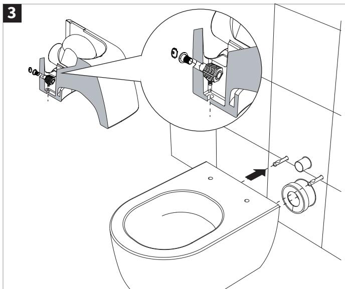
Place the toilet upside down and assemble the fixing kit on the toilet installation holes ensuring a tight fit. The grub screws should be facing up, so they can be accessed through the toilet seat holes. Place the toilet on the fixings.
