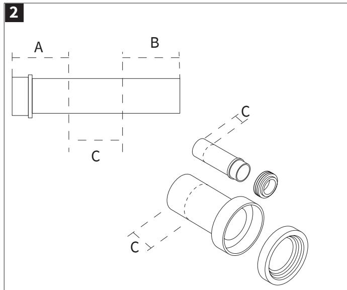
Push the inlet as far as possible into the toilet and mark the distance on the pipe. Measurement A. Then push the inlet into the concealed cistern as far as possible and mark the distance on the pipe. Measurement B. Measure the distance between both marks. Measurement C. Finally, cut measurement C off the end of the inlet pipe before securing the toilet to the wall. Follow the manufacturer's guidelines for applying grease to the seals
