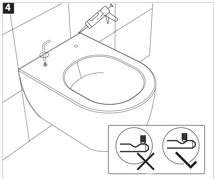
Secure the toilet to the concealed cistern and wall by tightening the grub screws to the bullet fixings. Apply a flexible sealant around the top and rear of the toilet as shown, leave to dry for 24 hours before use.
