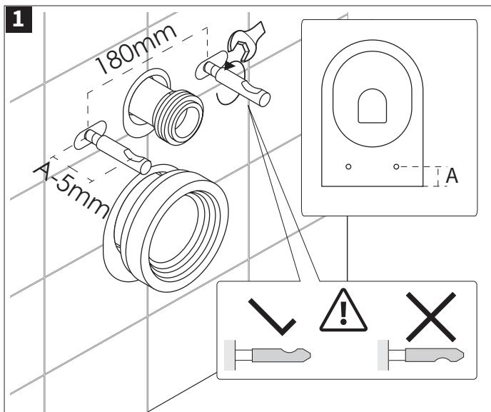
Follow the manufacturer's instructions for the installation of the concealed cistern selected, ensuring the fixing points match the width of the wall hung toilet. Measure distance A and reduce the depth of the bullet fixings by 5mm to ensure a tight grip against the wall surface. Make sure the bullet fixings are facing up.
