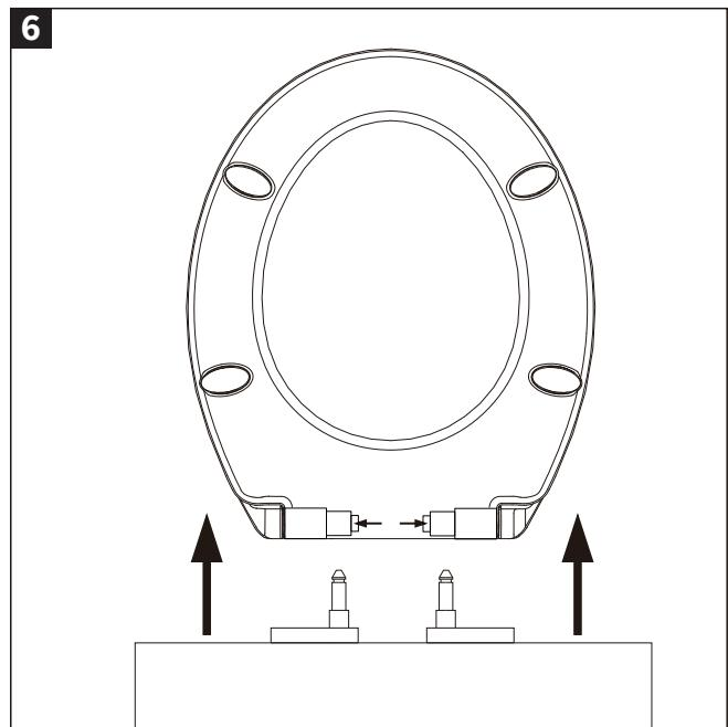
To remove the seat press the quick release button and lift off.
