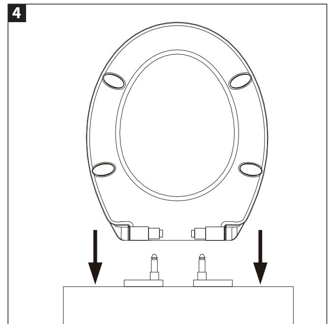
Before attaching the seat, move the mounting base so that the posts align with holes in the back of the seat. Once aligned, carefully lower the seat (holes) onto the mounting post.
