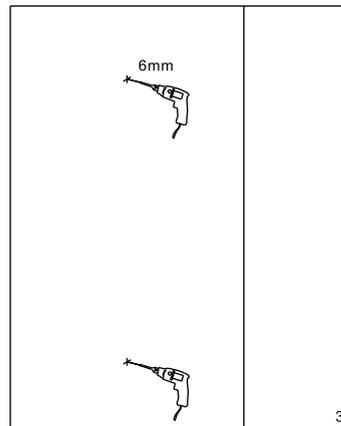
3. Drill two fitting holes by using a 6mm masonry drill bit.
