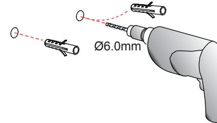
Using a 6mm drill bit, drill holes on the marked positions. Insert the rawl plugs into the drilled holes.
