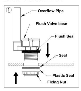
Insert flush valve base and flush seal through the tank flush hole. Tighten with the fixing nut, clamping the seals in place.
