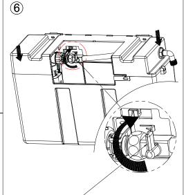
Adjust the flexible pipe to make sure the insulating valve is facing the front of the tank.
