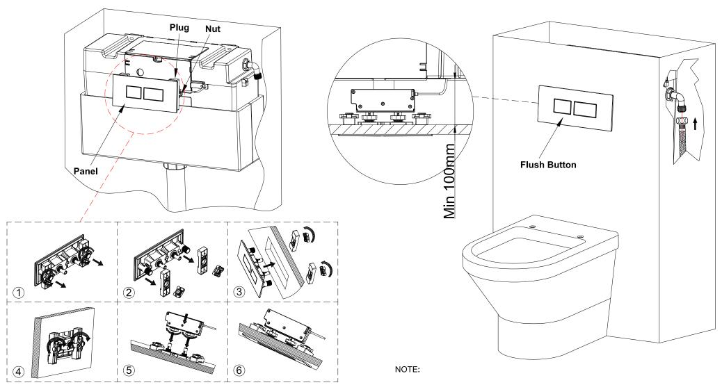
5. Remove the flush button by pressing down on the spring clip. Unscrew the fixing nut and insert the flush button through the cabinet hole. Tighten the flush button with the fixing nut clamping the cabinet between button and nut. From inside press down on the spring clip and insert the box onto the flush button. Make sure that the spring clip is engaged. If not press again. Connect the water supply to the inlet elbow.
