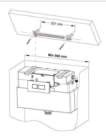
2. Note the minimum width required for this cistern is 560mm.
