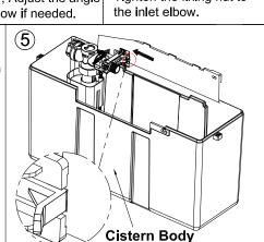
Clamp the Inlet Valve base to the cistern body.
