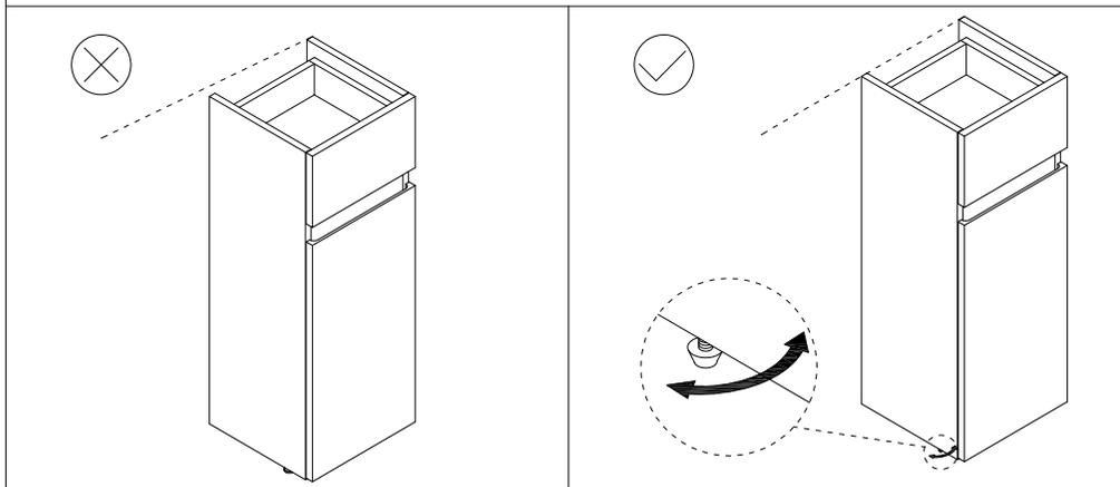
• Fix the cabinet onto the wall.
