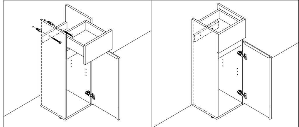
• Check the door for level. If not, please adjust the screw on the hinge.
