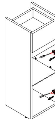
3: Attach the two hinge bases onto the opposite side panel in the right position as shown in the below diagram.
