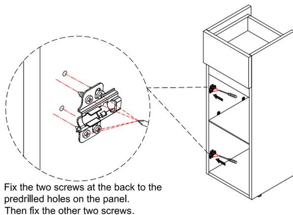
4: Reattach the door to the carcass, and insert parts A.
