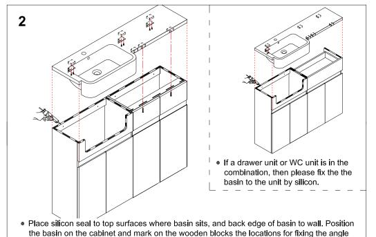
Apply a bead of silicone to hold the basin in position and to prevent water collecting between
