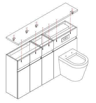
• Depending on your furniture combination use the brackets and fixing screws to secure the worktop as shown in the above diagram.
