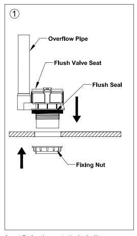
Insert flush valve seat attached with flush seal into tank flush hole, then screw up the fixing nut.
