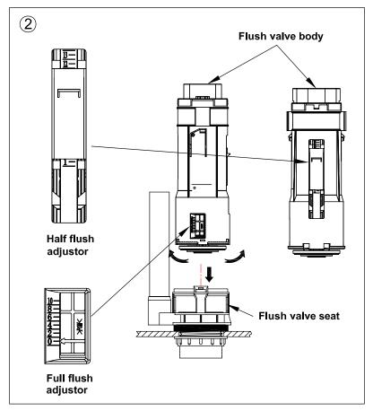
Insert flush valve body into flush valve seat, rotate it until it fixes onto the clip.
