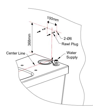
**1:** With the pan fixed into position, draw the water supply connector out of the pan through the access hole on the pan.
