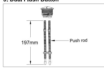
Screw the push rods out of the button, and cut the push rods to a length of 197mm as shown in the diagram on the left hand side.
