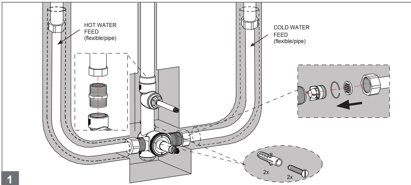
The valve should be installed in accordance with the water bye-laws. For further details refer to the latest copy of Water Bye-laws guide or your local water authority.
