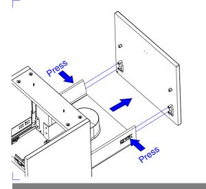
Press both blue buttons to release the drawer front.
