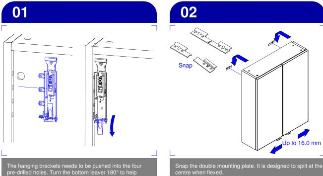
Measure and fit the brackets to the wall. IMPORTANT - The wall fixings are not supplied. Use the correct fixings to suit the wall construction.
