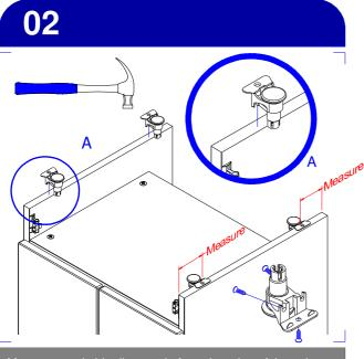
Measure a suitable distance in from the edge of the unit. The distance will vary depending upon the units depth. Position the foot as shown and knock the plate with a hammer to secure the foot to the side panel. Three additional screws can be used to secure in place. 03
