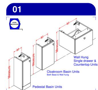
Determine the height of the unit required, taking into account the basin height when fitted. Mark the position of the units to the wall. The dimensions are to the outer edges of the unit carcase as shown.
