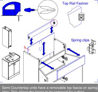
clips. This allows the fascia to be removed for cutting. Semi-Countertop &150w units have a removable 8mm back panel to allow for scribing. The top rail must be removed to allow the back to slide out.
