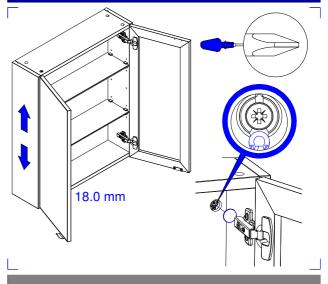
Remove the round cover cap from both holes. Turn the screw highlighted using a Philips No 2  $\emptyset$  6.0 or a Pozidrive No 2  $\emptyset$  6.0 screw driver. Anti-clockwise - Lower the cabinet Clockwise - Higher the cabinet
