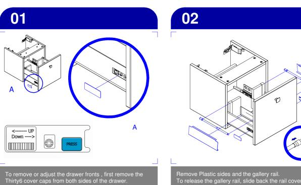
Remove Plastic sides and the gallery rail. To release the gallery rail, slide back the rail covers, and unhook from the rail front fixing. ( as shown in the detail ) This will reveal the drawer front adjustment controls and the blue drawer front removal button.
