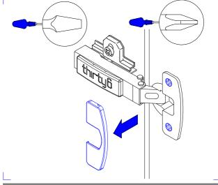
To remove the door only, the hinge cup cover cap needs to be gently eased away using a small thin
