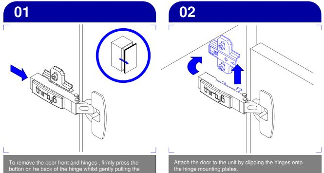
Attach the door to the unit by clipping the hinges onto the hinge mounting plates.
