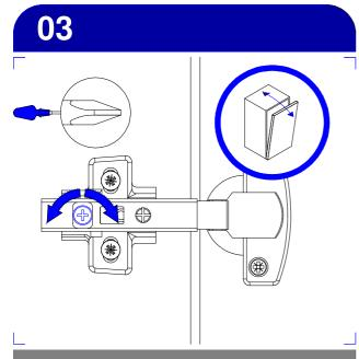
To adjust the door front back and fourth, Turn the screw shown clockwise/anti-clockwise.
