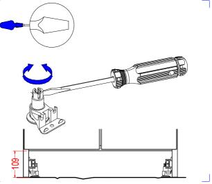
If the plinth is removed, the unit can be height adjusted by hand or flat headed screwdriver.
