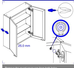
Remove the round cover cap from both holes. Turn the screw highlighted using a Philips No 2  $\emptyset$  6.0 or a Pozidrive No 2  $\emptyset$  6.0 screwdriver. Anti-clockwise - Loosen from the wall Clockwise - Tighten to wall
