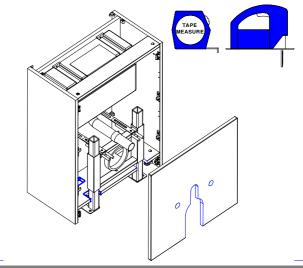
Remove the front panel and use any templates supplied with the WC pan to cut or drill the front panel.
