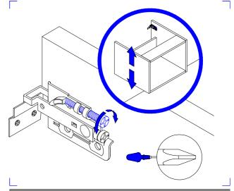
Adjust the height and level of the unit by turning the upper screw.
