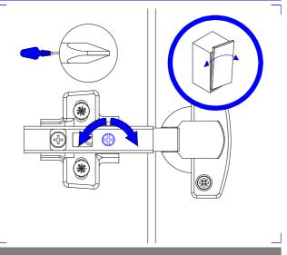
To adjust the door front horizontally, Turn the screw shown clockwise/anti-clockwise.
