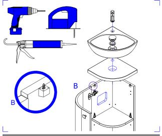
Check and mark the position of the basin on the top. Double check before drilling and cutting. Cut the panels and then seal any cut edges to stop water getting into the chipboard. Fit the top and basin. Seal around the basin with silicone sealant and smooth.
