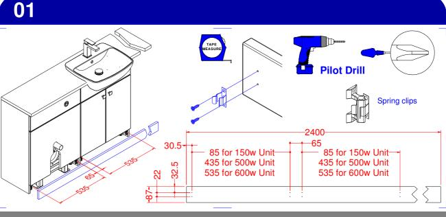
When fitted units are joined in a run the plinth will need to be fixed to the units using the spring clips provided.
