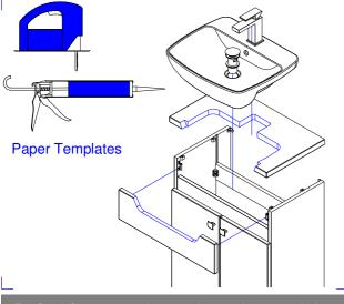
For Semi-Countertop units., use the templates supplied to mark out the top and fascia. Double check before cutting. Cut the panels and then seal any cut edges to stop water getting into the chipboard. Fit the top and basin. Seal around the basin with silicone sealant and smooth.
