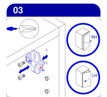
To change the handing of the door unscrew the hinge mounting plate. Swap the cover caps from the opposite side.
