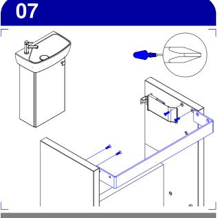
On the Cloakroom Units the Front Rail needs to be removed to be able to access the cover plate.
