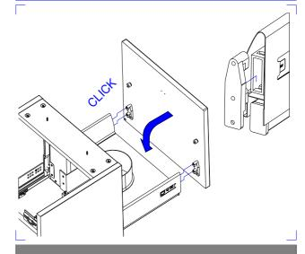
To re-fit the drawer front, position the drawer front hook bracket inside the curved drawer box side panel The hooks should CLICK into place into the square holes in the runner.
