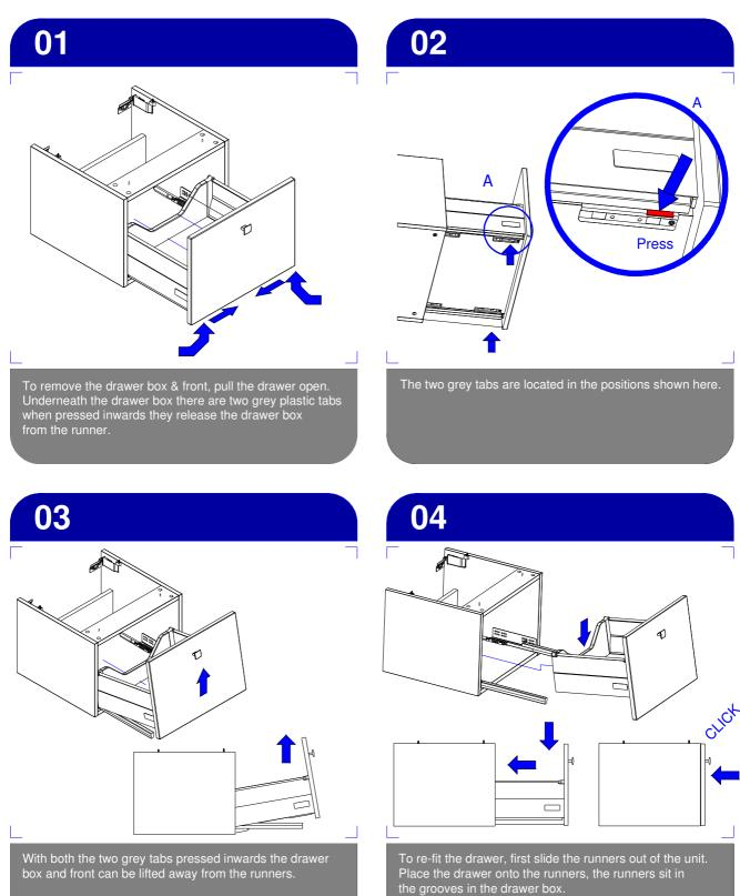
the grooves in the drawer box. Push the drawer fully into the unit. The drawer will CLICK into place.
