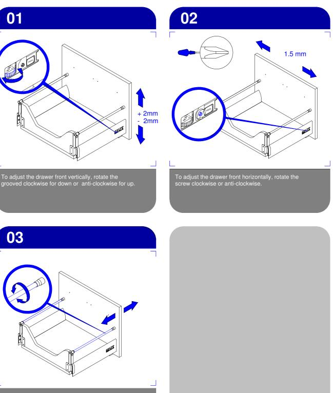
To adjust the drawer front back & forth, twist the rails clocckwise or anti-clockwise.
