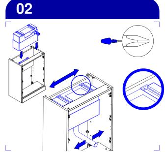
Once the cistern is slotted onto the bracket , it can be moved sidways to position the down pipe into the desired
