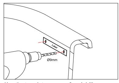
Use the template on page 2 and drill the 4 holes accordingly.
