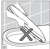
**NOTE:** Only install and remove the seat and cover at an angle of  $90\pm5^\circ$ . Failure to do this will result in damage to the seat and cover.
