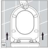
10. To remove the seat and cover at an angle of 90±5°.
