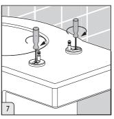
7. Fully tighten the fixings.
