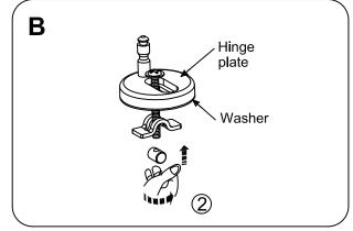
② Insert the pan fixing bolt through the hinge plate and the washer.
