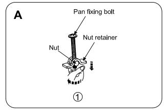
① Unscrew the nut from the pan fixing bolt. Remove the nut retainer from the pan fixing bolt.
