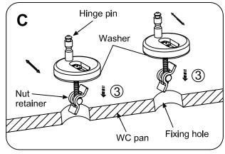
(3) Flip the nut retainer into a vertical position and insert through the pan fixing hole as shown in Figure C 3.
