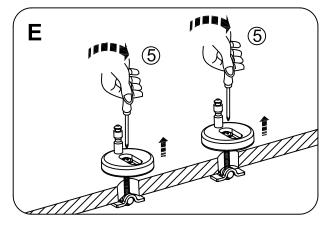
(5) Whilst holding the hinge plate and clamping the nut retainer to the pan, tighten the pan fixing bolt using a screw driver - as shown in Figure E 5. As the pan fixing bolt tightens the hinge plate will lower until fitting tightly to the pan.
