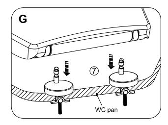
The Attach the WC seat onto the hinge pins as shown in Figure G.7.
