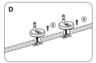
When inserted, gently shake the pan fixing bolt so that the nut retainer turns to a horizontal position. Once the nut retainer is horizontal, raise the hinge plate and pan fixing bolt so that the nut retainer is firmly held in position by the underside of the ceramic pan- as shown in Figure D 4.
