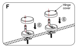
Gently tighten the pan fixing bolt, then fix the seat on to the hinge pins and check if the adjustment of the hinge plate is correct. If the wc seat fits correctly remove the seat and do a final firm fix of the pan fixing bolts to prevent the seat moving or working loose.
