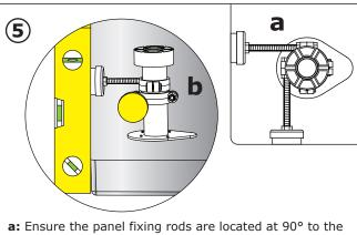
**a:** Ensure the panel fixing rods are located at 90° to the edge of the tray as shown above.
