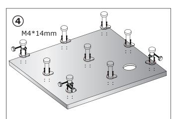
Screw the feet in position with the screws provided. Ensure that the foot that has panel fixing rod attached, is placed edges where the panels will be mounted.
