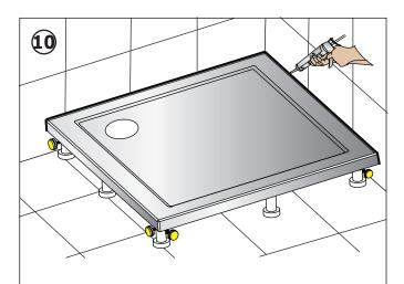
Tile the wall and seal joints with an anti fungal silicone sealant and allow to set.
