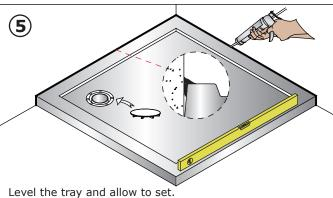
When shower tray is set remove the remainder of the protective plastic film and connect the waste pipe and
