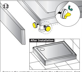
Remove the protective cover from the adhesive tape. First fix the rebated panel pushing it firmly on to the adhesive pads. Then fix the remaining panel in the same manner.
