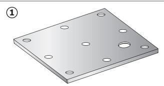
Turn the tray over and use the cardboard packaging as a protective mat. Note the circles that have been marked to indicate feet position. The symbol  $\bigoplus$  indicates where you should fix the feet with the panel fixing rod, but for the symbol  $\bigoplus$  you will only use three of these positions and the fourth would be supplemented with a foot without the panel fixing rod.
