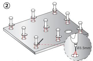
Using the foot as a guide mark with a pencil the fixing hole positions, and then using a 3.5 diameter bit drill to a maximum depth of 5mm. DO NOT OVER DRILL PAST THE 5MM DEPTH.
