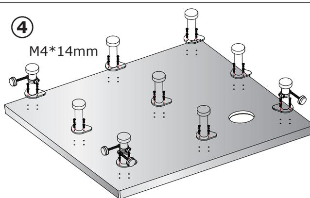
Screw the feet in position with the screws provided. Ensure that the foot that has panel fixing rod attached, is placed edges where the panels will be mounted.
