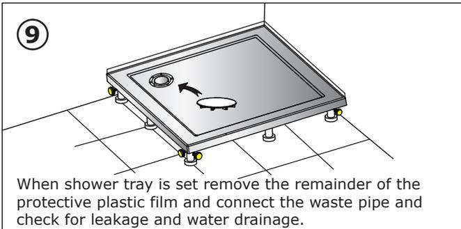
When shower tray is set remove the remainder of the protective plastic film and connect the waste pipe and check for leakage and water drainage.
