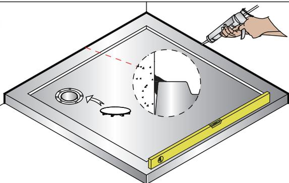
Level the tray and allow to set. When shower tray is set remove the remainder of the protective plastic film and connect the waste pipe and check for leakage.
