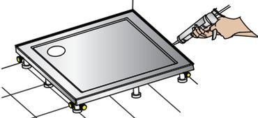
\* If the 'easyseal' water sealing strip is not installed, please seal joints between tray and wall with an anti fungal silicone sealant and allow to set.
