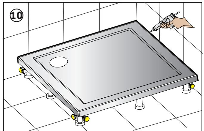
Tile the wall and seal joints with an anti fungal silicone sealant and allow to set.
