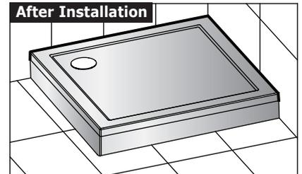
Remove the protective cover from the adhesive tape. First fix the rebated panel pushing it firmly on to the adhesive pads. Then fix the remaining panel in the same manner.
