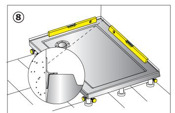
Ensure the 'easyseal' water sealing strip is flat to the wall. Place the tray into position and level both ways using the legs. After the tray has been levelled adjust all the inner feet to stabilise the tray. When level fix these legs to the floor with silicon sealant or 'no more nails' type adhesive.
