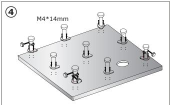
Screw the feet in position with the screws provided. Ensure that the foot that has two panel fixing rods attached, is placed in the corner where the panels will
