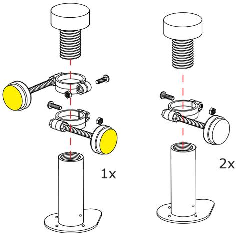
Assemble the panel fixing rods to the feet.
