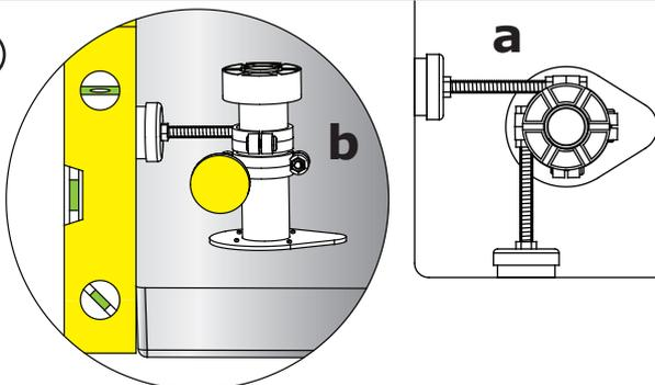
**a:** Ensure the panel fixing rods are located at 90° to the edge of the tray as shown above.
