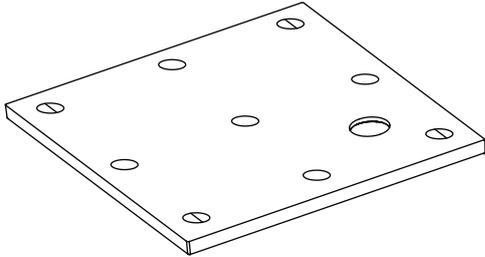
Turn the tray over and use the cardboard packaging as a protective mat. Note the circles that have been marked to indicate feet position. The symbol  $\ominus$  indicates where you should fix the feet with the panel fixing rod, but for the symbol  $\oplus$  you will only use three of these positions and the fourth would be supplemented with a foot without the panel fixing rod.
