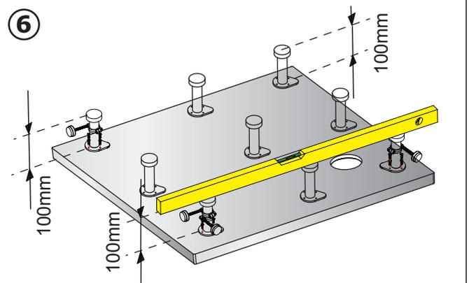
When all of the feet have been fitted, the feet in the corner positions should be adjusted to 100mm.
