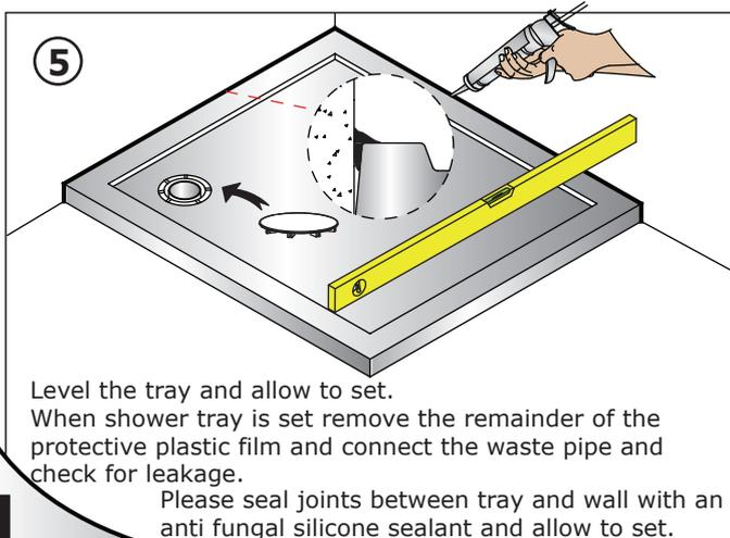
Level the tray and allow to set. When shower tray is set remove the remainder of the protective plastic film and connect the waste pipe and check for leakage. Please seal joints between tray and wall with an anti fungal silicone sealant and allow to set.
