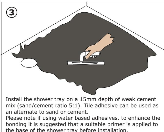
Install the shower tray on a 15mm depth of weak cement mix (sand/cement ratio 5:1). Tile adhesive can be used as an alternate to sand or cement. Please note if using water based adhesives, to enhance the bonding it is suggested that a suitable primer is applied to the base of the shower tray before installation.
