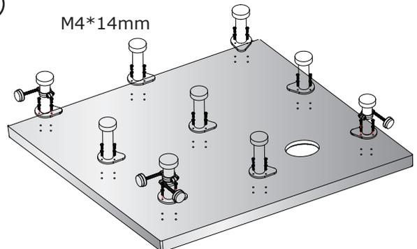
Screw the feet in position with the screws provided. Ensure that the foot that has two panel fixing rods attached, is placed in the corner where the panels will meet.
