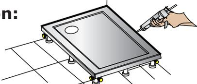
\* If the 'easyseal' water sealing strip is not installed, please seal joints between tray and wall with an anti fungal silicone sealant and allow to set.
