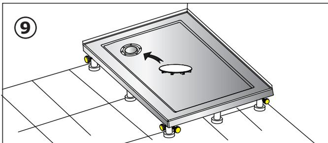
When shower tray is set remove the remainder of the protective plastic film and connect the waste pipe and check for leakage and water drainage.
