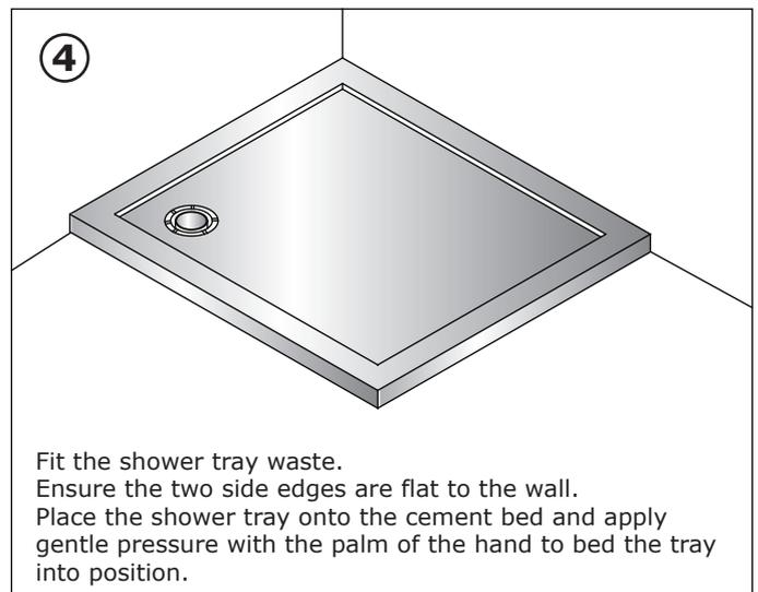
Fit the shower tray waste. Ensure the two side edges are flat to the wall. Place the shower tray onto the cement bed and apply gentle pressure with the palm of the hand to bed the tray into position.
