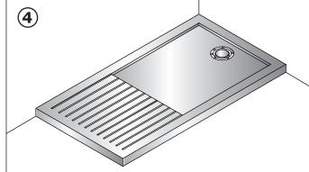
Fit the shower tray waste. Ensure the two side edges are flat to the wall. Place the shower tray onto the cement bed and apply gentle pressure with the palm of the hand to bed the tray into position.
