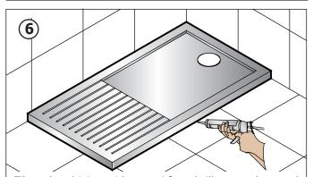
Tile and seal joints with an anti fungal silicone sealant and allow to set.
