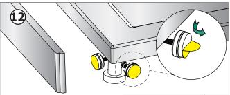
Remove the protective cover from the adhesive tape. First fix the rebated panel pushing it firmly on to the adhesive pads. Then fix the remaining panel in the same manner.
