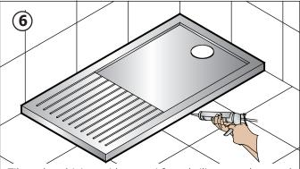
Tile and seal joints with an anti fungal silicone sealant  $% \left( 1\right) =\left( 1\right) +\left( 1\right) +$
