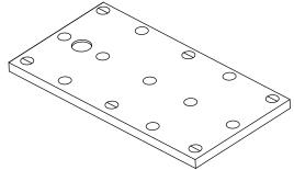
Turn the tray over and use the cardboard packaging as a protective mat. Note the circles that have been marked to indicate feet position. The symbol ⊖ indicates where you should fix the feet with the panel fixing rod, but for the  $\operatorname{symbol} igoplus \operatorname{you}$  will only use four of these positions and the other two would be supplemented with the feet without the panel fixing rod.
