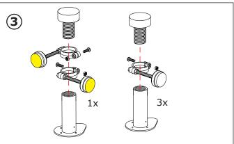
Assemble the panel fixing rods to the feet.
