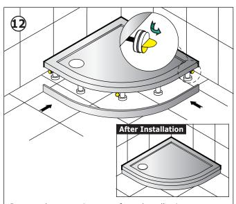
Remove the protective cover from the adhesive tape. Fix the panel pushing it firmly on to the adhesive pads.
