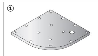
Turn the tray over and use the cardboard packaging as a protective mat. Note the circles that have been marked to indicate feet position. The symbol  $\bigoplus$  indicates where you should fix the feet with the panel fixing rod.
