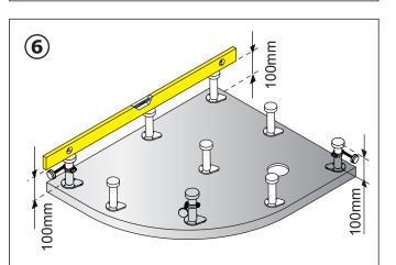
When all of the feet have been fitted, the feet in the corner positions should be adjusted to 100mm.
