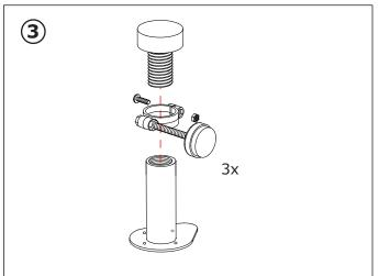
Assemble the panel fixing rods to the feet.
