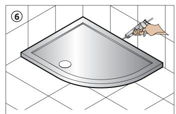
Tile and seal joints with an anti fungal silicone sealant and allow to set.
