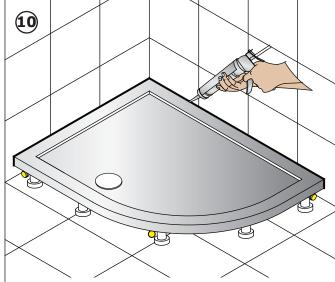
Tile the wall and seal joints with an anti fungal silicone sealant and allow to set.
