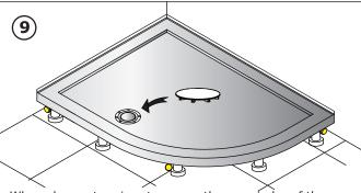
When shower tray is set remove the remainder of the protective plastic film and connect the waste pipe and check for leakage and water drainage.
