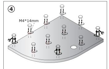
Screw the feet in position with the screws provided. Ensure that the feet that have panel fixing rod attached, are placed around the curved edge where the panels will meet.
