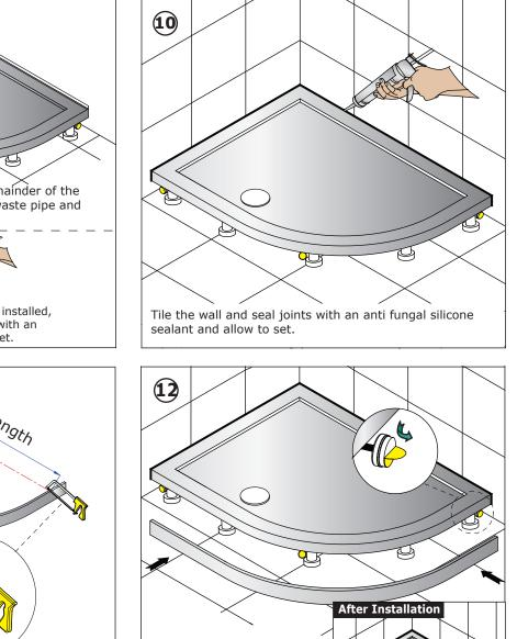
Remove the protective cover from the adhesive tape. Fix the panel pushing it firmly on to the adhesive pads.
