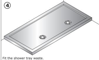
Ensure the two side edges are flat to the wall. Place the shower tray onto the cement bed and apply gentle pressure with the palm of the hand to bed the tray into position.
