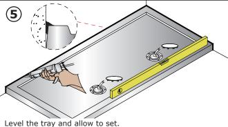
When shower tray is set remove the remainder of the protective plastic film and connect the waste pipe and check for leakage.
