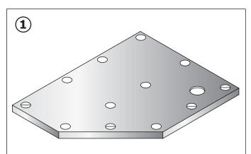
Turn the tray over and use the cardboard packaging as a protective mat. Note the circles that have been marked to indicate feet position. The symbol  $\bigoplus$  indicates where you should fix the feet with the panel fixing rod.
