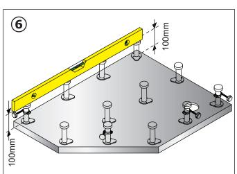
When all of the feet have been fitted, the feet in the corner positions should be adjusted to 100mm.
