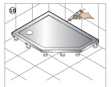
Tile the wall and seal joints with an anti fungal silicone sealant and allow to set.
