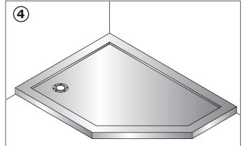
Fit the shower tray waste. Ensure the two side edges are flat to the wall. Place the shower tray onto the cement bed and apply gentle pressure with the palm of the hand to bed the tray into position.
