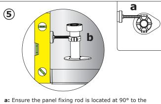
**a:** Ensure the panel fixing rod is located at 90° to the edge of the tray as shown above.
