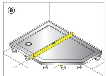
Ensure the 'easyseal' water sealing strip is flat to the wall. Place the tray into position and level both ways using the legs. After the tray has been levelled adjust all the inner feet to stabilise the tray. When level fix these legs to the floor with silicon sealant or 'no more nails' type adhesive.
