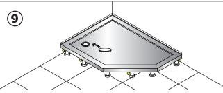
When shower tray is set remove the remainder of the protective plastic film and connect the waste pipe and check for leakage and water drainage.
