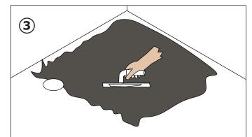
Install the shower tray on a 15mm depth of weak cement mix (sand/cement ratio 5:1). Tile adhesive can be used as an alternate to sand or cement.
