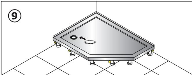
When shower tray is set remove the remainder of the protective plastic film and connect the waste pipe and check for leakage and water drainage.
