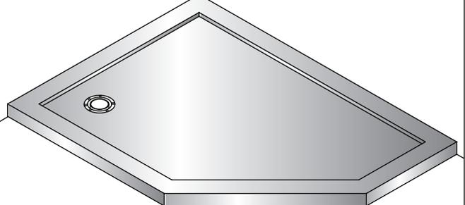
Fit the shower tray waste. Ensure the two side edges are flat to the wall. Place the shower tray onto the cement bed and apply gentle pressure with the palm of the hand to bed the tray into position.
