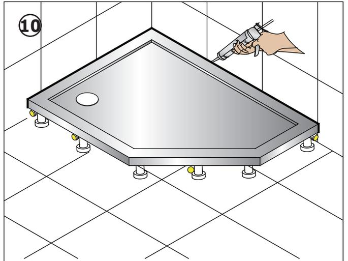
Tile the wall and seal joints with an anti fungal silicone sealant and allow to set.
