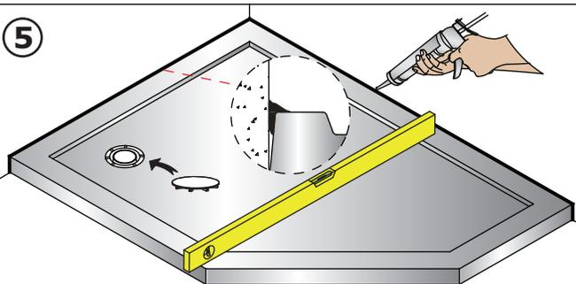
Level the tray and allow to set. When shower tray is set remove the remainder of the protective plastic film and connect the waste pipe and check for leakage.
