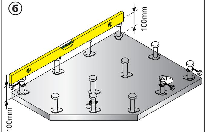
When all of the feet have been fitted, the feet in the corner positions should be adjusted to 100mm.
