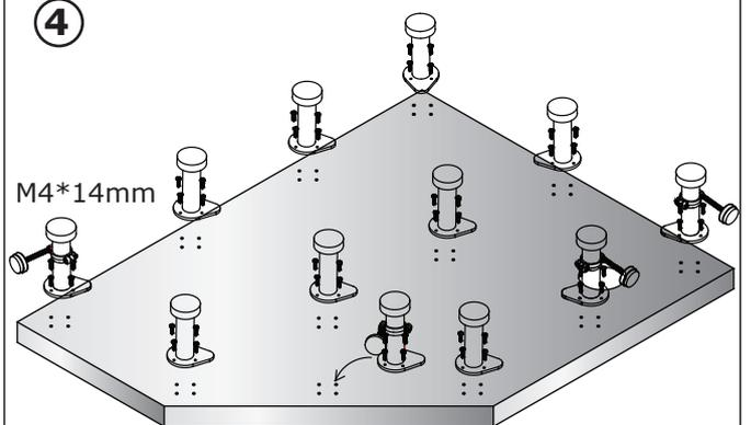
Screw the feet in position with the screws provided. Ensure that the feet that have panel fixing rod attached, are placed around the bended edge where the panel will meet.
