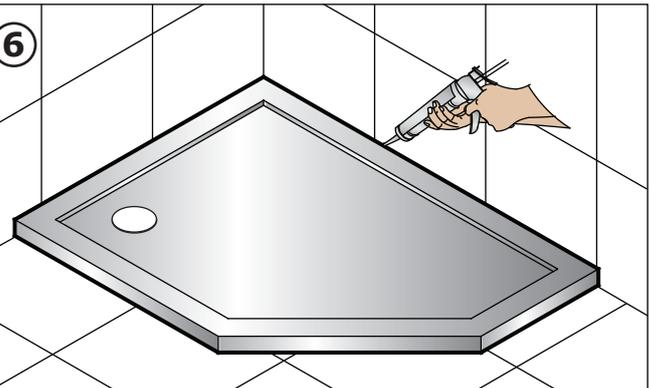
Tile and seal joints with an anti fungal silicone sealant and allow to set.
