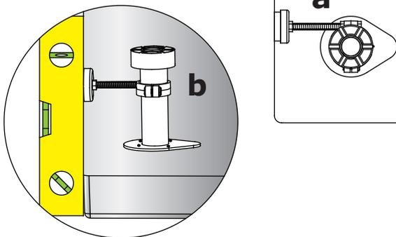
**a:** Ensure the panel fixing rod is located at 90° to the edge of the tray as shown above.
