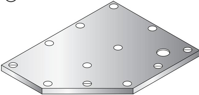
Turn the tray over and use the cardboard packaging as a protective mat. Note the circles that have been marked to indicate feet position. The symbol  $\ominus$  indicates where you should fix the feet with the panel fixing rod.
