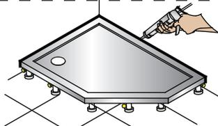
\* If the 'easyseal' water sealing strip is not installed, please seal joints between tray and wall with an anti fungal silicone sealant and allow to set.
