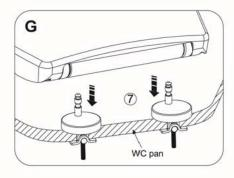
7 Attach the WC seat onto the hinge pins as shown in Figure G 7.
