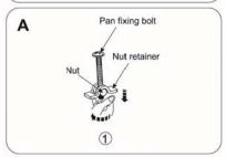
Unscrew the nut from the pan fixing bolt. Remove the nut retainer from the pan fixing bolt.
