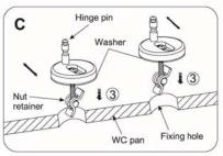
Flip the nut retainer into a vertical position and insert through the pan fixing hole as shown in Figure C 3.
