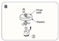
(2) Insert the pan fixing bolt through the hinge plate and the washer.
