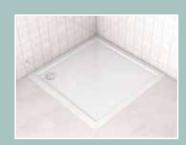
The low 35mm height allows the tray to be sunk into the floor so that the upper surface is level with the floor. The framed rim still allows good water retention to avoid water escape, especially when combined with the self cleaning Vortex high flow shower waste (which clears up to 30 litres of water per minute).
